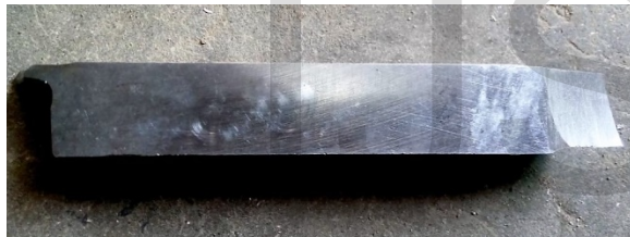
Figure 2 : HSS Tool geometry with positive rake angle
